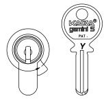
Function with duplo key ensures full functionality (bolt and latch activation)
